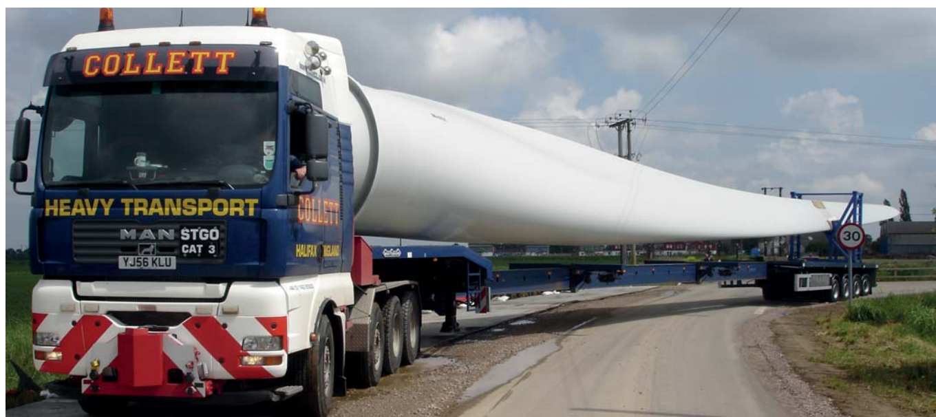
A Collett & Sons lorry transporting a turbine blade to site Photo: Collett & Sons
